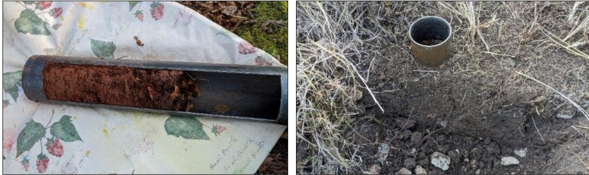
Figure 6. Soil sampling for ^{137}\text{Cs} analysis: core sampling with 5 cm interval slicing (left); cylinder sampling from an opened soil profile at successive 5 cm depths (right)
